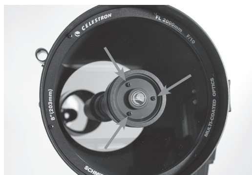
Secondary Mirror Collimation Adjustment Screws
